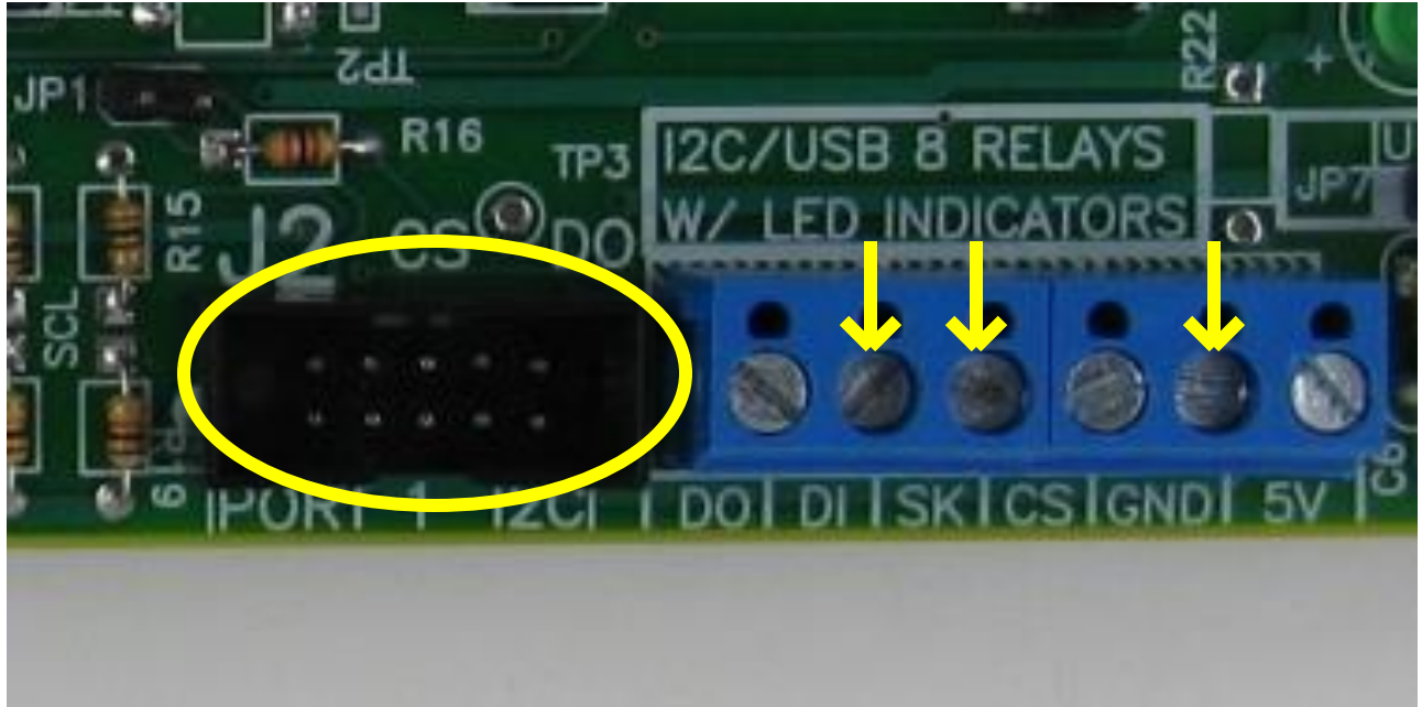
Figure 4: Ribbon connector port J2, and the alternative terminal block pins needed for I 2 C communications.
