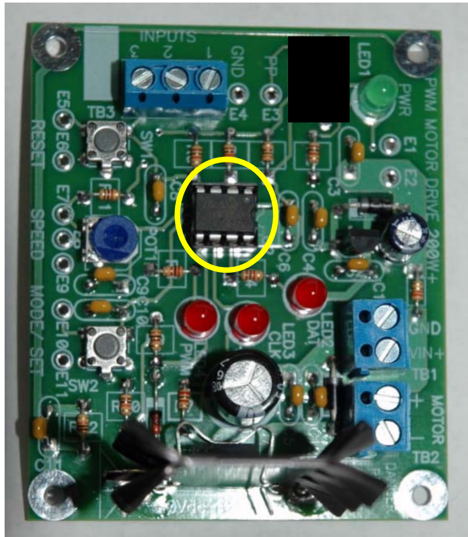
Figure 20: Board with socket and processor installed.
