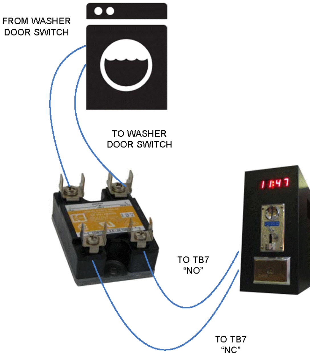
Figure 7: Wiring Diagram for A/C Appliance Hook-Up
